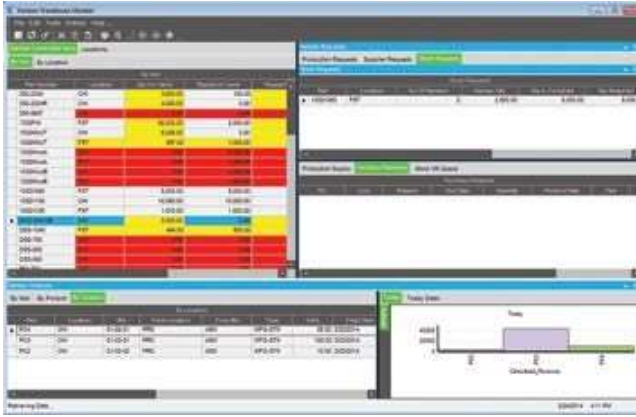
Manage electronic queues for Kanban control with the Kanban Monitor. Optionally display on the plant floor information about current Kanban records in a dashboard format.
